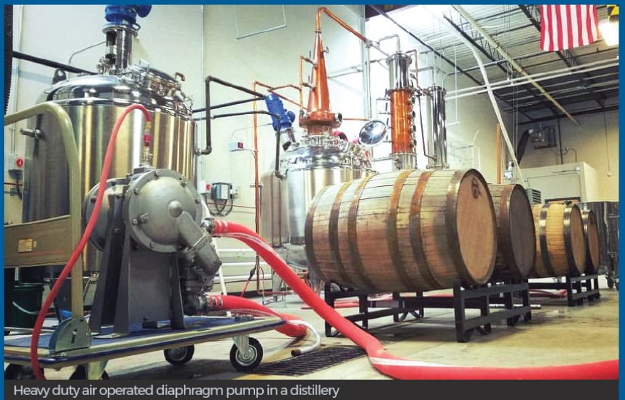
Heavy duty air operated diaphragm pump in a distillery
