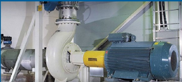
Heavy-duty centrifugal pump on 12% paper stock
