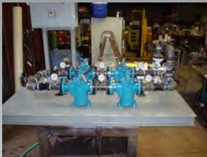
Centrifugal pump system with two stage redundant afterfilters. Skid computer model at left, finished system at right.
