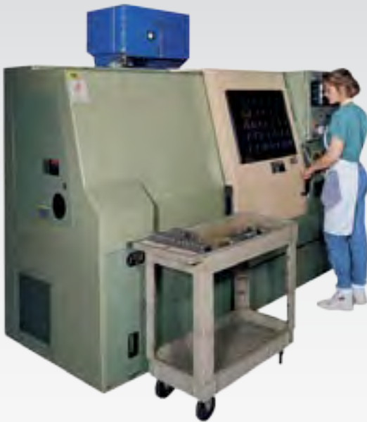
Machine-mounted coolant mist collector on a CNC machining center.
