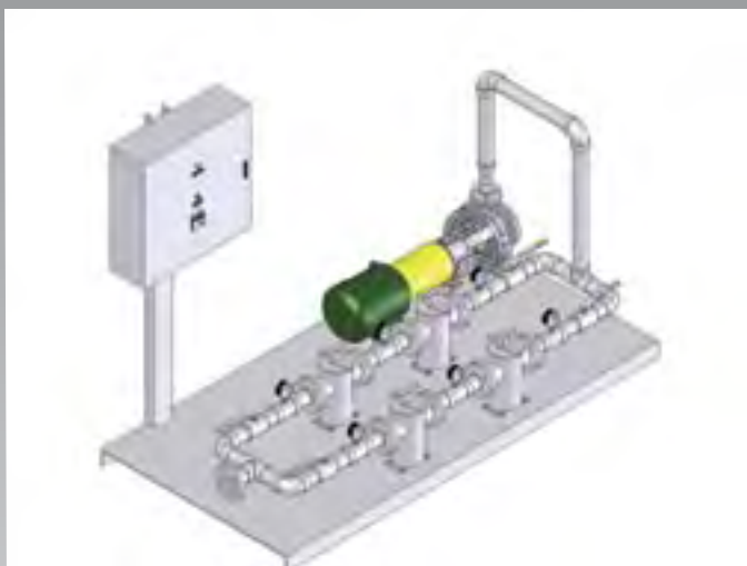
Centrifugal pump system with two stage redundant afterfilters. Skid computer model at left, finished system at right.
