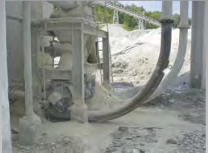
Rotary airlocks with wear-back elbows conveying lime kiln dust at 450 degrees Fahrenheit.
